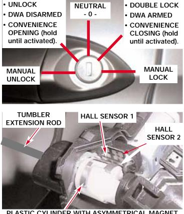
PLASTIC CYLINDER WITH ASYMMETRICAL MAGNET (Shown in the Lock Position)
